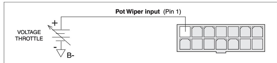
The PotHigh and PotLow parameters are used to set the voltage range of these throttles. If the pot wiper voltage is higher than the programmed PotHigh
