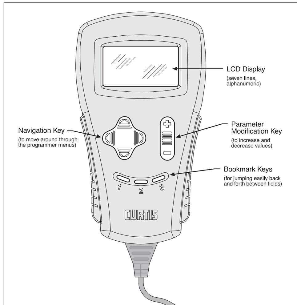
information from the controller. For experimenting with settings, the programmer can be left plugged in while the vehicle is driven.
