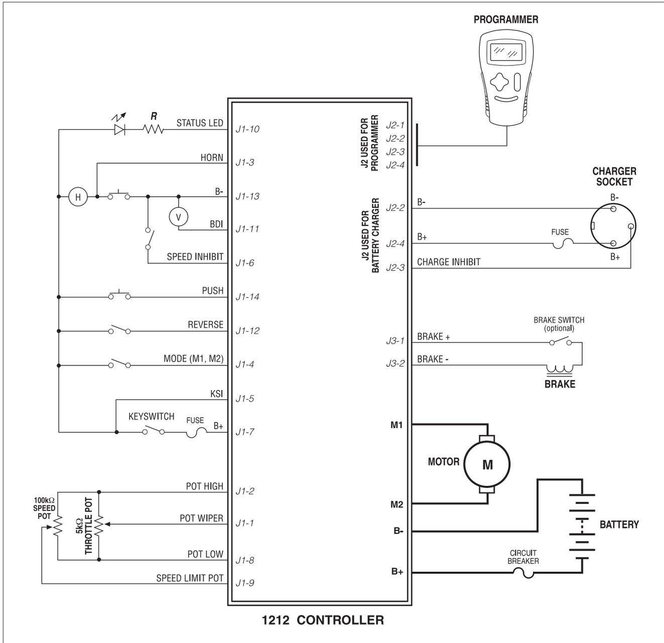
Fig. 3 Standard wiring configuration, Curtis 1212 controller.
