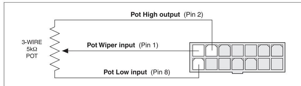
For wigwag, inverted wigwag, and unipolar applications, the pot can be correctly centered within the controller's neutral band by using the throttle autocalibration feature (see page 18).
